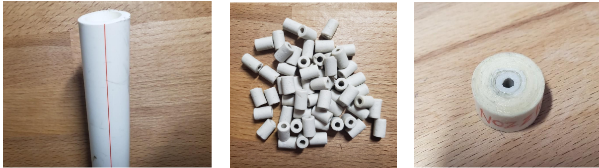
Fig 3.14 (a) PPR tube (b) ceramics tubes (c) a nozzle made of ceramic core, tape and glue
